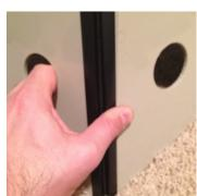
Ensure the top screw is aligned as shown in photo. Tighten the screw clockwise until you feel the whole pyramid tighten up. *Tip: Do not over tighten as screw may break.*
